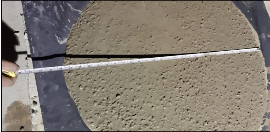
*FIGURA 60. ASPECTO DE LA MEZCLA AUTOCOMPACTABLE DE REFERENCIA REALIZADA EN LA FASE EXPERIMENTAL, DESPUÉS DEL ENSAYO DE ESCURRIMIENTO*
