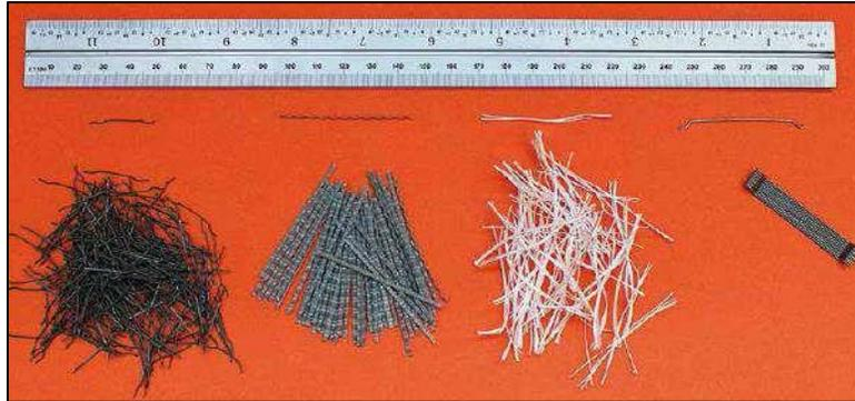
FIGURA 13. DIFERENTES TIPOS DE FIBRAS (DE ACERO Y SINTÉTICAS).
