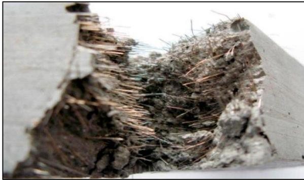
FIGURA 5. CONCRETO REFORZADO CON FIBRAS.
